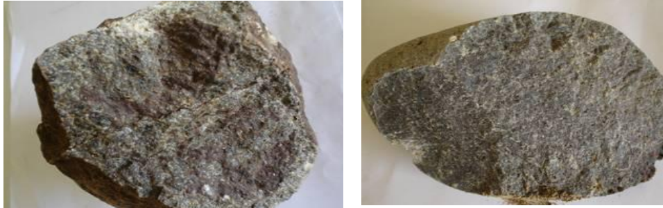
FIGURES N° 2 and 3. Basalts of fine texture constituted of numerous irregularly distributed small crystals located in a mass of even finer crystals or glass.
